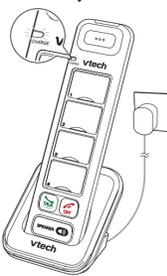
Once you have installed the battery and placed the handset in the charger, the **CHARGE** light indicates the battery status (see the table below).
